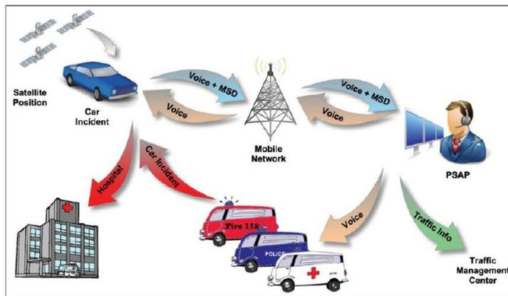
**Figure 1: The operational cycle of eCall**
